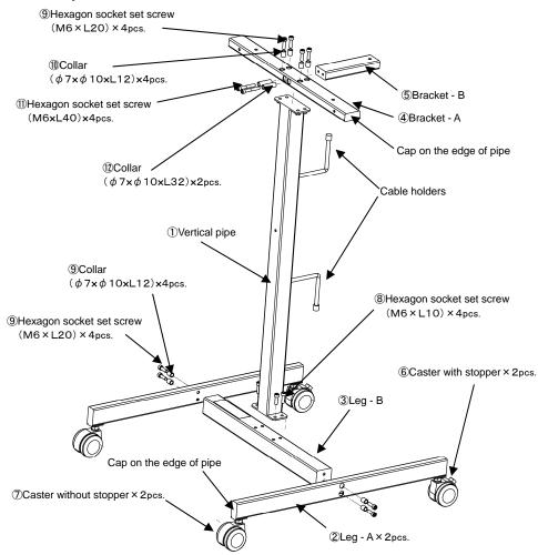
\* If you drop the collar into the pipe while assembling the stand, you can take it out by removing the cap on the edge of pipe.
